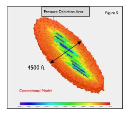
The pressure change in the fractures at the end of the 10 year prediction period for the two models are shown in Figures 5 and 6. The cells shown in these figures represent areas of the model where the pressure has changed by greater than 200 psia in the fractures from initial conditions at the time shown. (Red areas are at near-initial pressure. Blue areas have experienced significant pressure reduction.) All other cells in the model are not shown.
