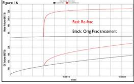
The SRV is shown in Figure 17. The incremental cumulative oil production over the base case (Figure 16) is significant. The cumulative water production is also significantly increased as the second frac treatment fluid volumes are produced, essentially during the first year after the refrac treatment. Actual re-frac data should be used to calibrate the model.
