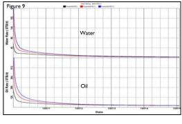
The production rate plot (Figure 9) for the first five years for each of the higher frac volume cases shows the rates are significantly higher in the first 2-3 years. Economic analysis will determine whether the cost of the larger fracture treatment is warranted by the increased rate and higher ultimate recovery (Figure 10).
