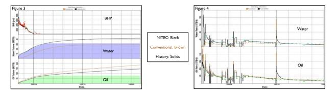
Figure 3 shows the cumulative water and oil production for the historical period and at the end of the 10 year prediction. The cumulative oil production for the prediction was
