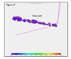
orientation is closer to being perpendicular to the principle stress direction than the original orientation; hence better communication is established with the natural fracture system.
