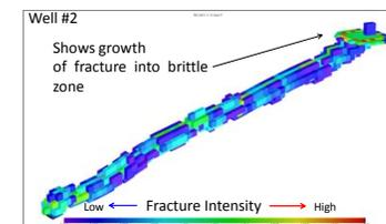
By generating the SRV with the hydraulic fracturing treatment it is possible to quantifiably predict how changes to the fracturing treatment will impact productivity
