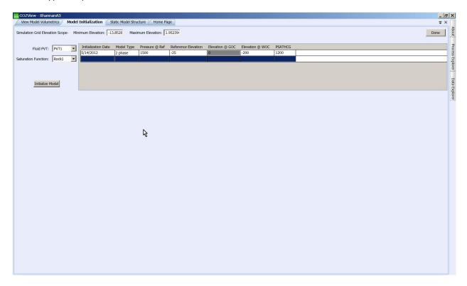
If the WOC is specified below the deepest elevation in the model there will not be a water leg (aquifer) in the model, but the model type is still 2-phase.
