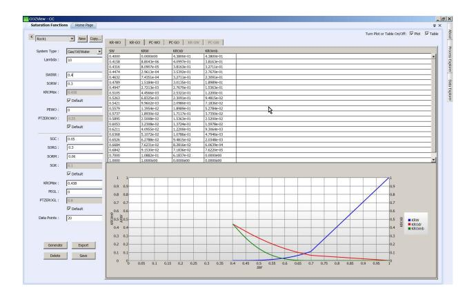
As noted above, the user can modify the shape of the individual saturation function curves with appropriate changes to endpoint parameters.
