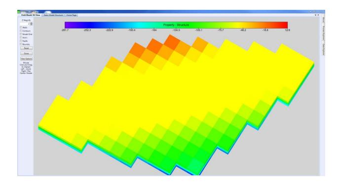
The initial 3D view will be a high angle representation of the surface with a vertical Z Magnification of 2. This Z magnification can be changed by the user.
