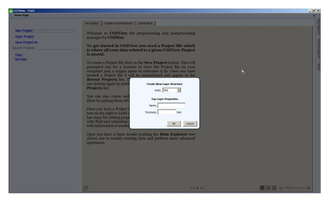
At any time after defining the *Top Layer Properties*, the user can save the model by clicking the **Save and Continue** button or the **Save and Quit** button. Periodic saving is suggested as the model is built. Leaving the *Static Model* area without saving may result in a loss of data.
