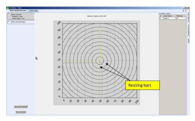
To the right and below the center of the interior circle are two *resizing bars* which allow the user to alter the shape of the contour surface. Movement of the *resizing bar* vertically with a left *click and drag* mouse operation, results in the figure below.
