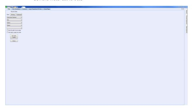
COZView has two options to set the scale for the Plots. (i) User can check the box "Use all wells to set scales". Selection of this box will automatically control the scales (X and Y axis) based on Property (Rates, Pressure, Cumulative, GOR and Water Cut) values for all wells. (ii) User is allowed to change the
