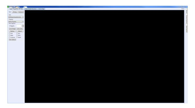
The menu in the **Select Property** box allows the user to select any of the formation properties previously input and saved. These reservoir properties are TVT NET (Net True Vertical Thickness), PHI Matrix (Matrix Porosity), Rock Compressibility, KX,KY and KZ (Permeability of matrix in X,Y and Z directions).
