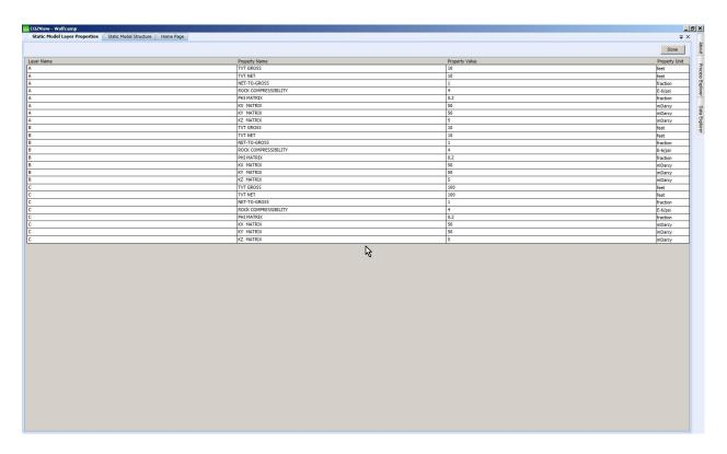
Property values are input by double clicking in the Property Value field and inputting the desired value. The property units for each property have defaulted to typical units. However, double clicking in the Property Unit field for a given property provides a dropdown menu for selection of alternative units.
