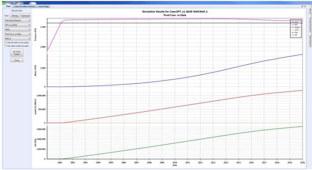
A unique functionality in COZView is the ability to assess a specific plot parameter value using the mouse. Placing the cursor on a specific plot trace and holding down the left button will display the value and date of the selected point. Continue holding down on the left mouse button and move the cursor to view other points on the same plot trace. The process can be repeated on other plot traces.
