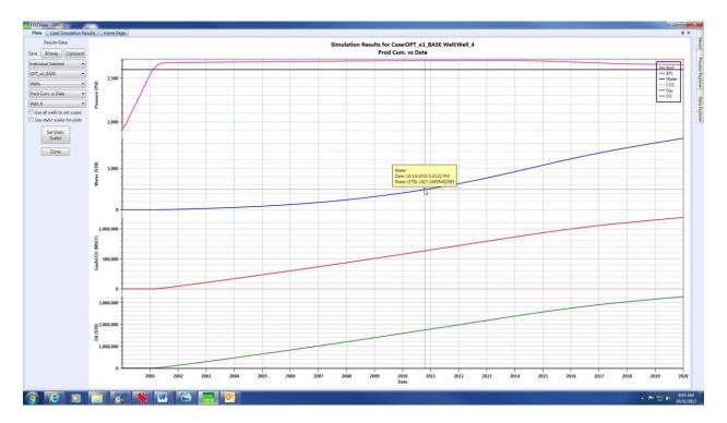
Any selected plot can be exported to a bitmap file for archiving by selecting the **Bitmap** button. Selection of the **Clipboard** button will place the plot image on the clipboard for pasting into a user selected document.
