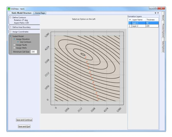
A right-click on a contour allows the user to assign a value to that contour. The user can assign contour values to any **two** contours. The implied contour interval calculated by the software will be used to assign values to the rest of the contours. Should the user wish to start over with the contour value assignment, a right-click on the contour and selection of *Reset All* is available.
