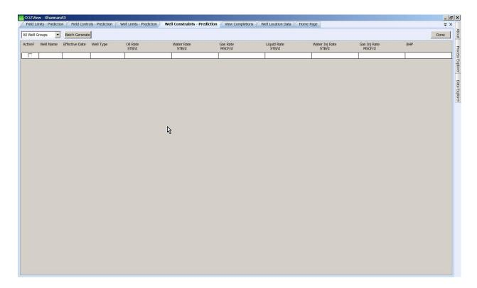
The *Well Constraints* menu identifies the Well type, desired production and injection rates and bottom hole flowing pressure for each well. A left-click on the blank row followed by a left-click in a data field provides either a drop down menu or the ability to input a value.
