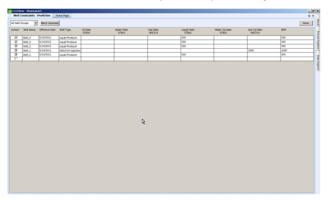
The simulator will initiate individual well production based on the greater of an assumed bottom hole flowing pressure of 14.7 psia or the user specified BHP. The well's production rate will be constrained by the well rates specified above.
