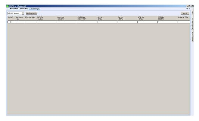
When a large number of wells are involved, the user may choose to use the **Batch Generate** button. The Batch Generate functionality allows quick assignment of parameter values to multiple wells.
