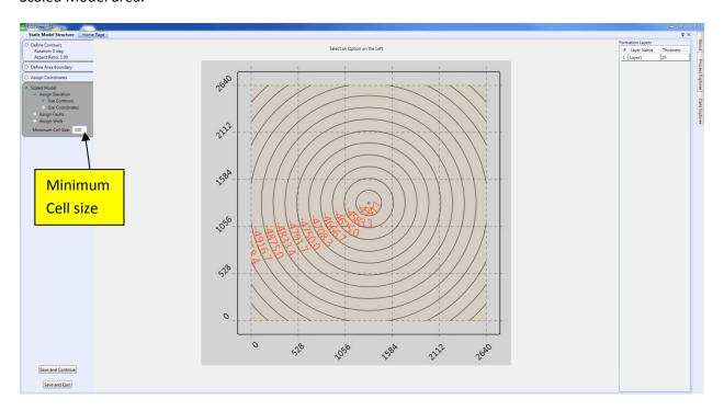
This should be done with caution. Reducing the minimum cell size will increase the number of total cells in the model, which will increase the simulation run time. This should only be done for the noted "small acreage" models. The minimum cell size is 220 ft. The maximum number of cells in the X- and Y-directions will not be allowed to exceed 100.
