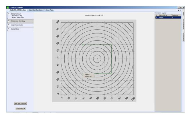
Individual boundary control points can be moved by a left-click and drag to a new location. If this is done after the coordinates of the boundary control point have been set, the coordinates for the moved-points must be re-defined.
