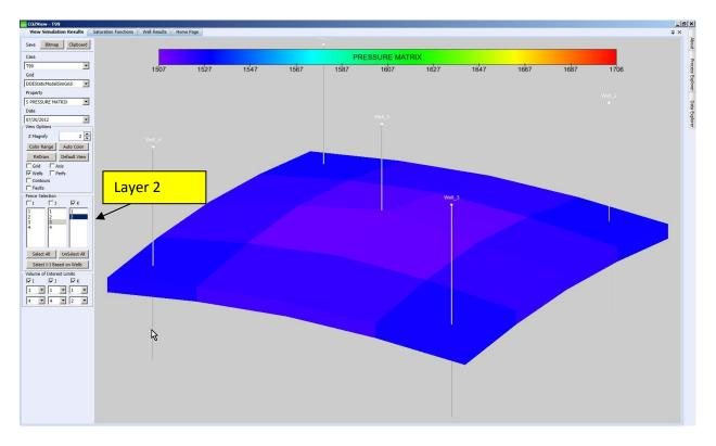
The range for the color scale can be changed by selecting the **Color Range** button. The maximum and minimum range values can be changed. This change will be applied to the current property only. It will not be saved upon selection of a different property.
