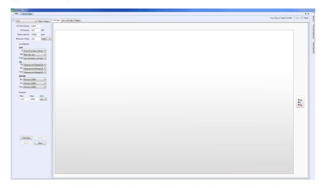
The user must then input appropriate values for the hydrocarbon gas (HC) *Gas Gravity, Oil Gravity, Water Salinity, Reservoir Temperature* and *Temperature Units*. At the bottom of the parameter panel, the minimum and maximum pressure range for the PVT values to be calculated must also be specified. The maximum pressure should be greater than any static or dynamic pressure the user expects to occur in the model during the simulation runs.
