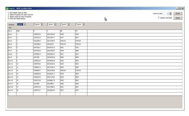
Each of the columns has a drop down menu from which the user must select a parameter in order to identify the column content. If the .csv file contains a header row(s), the user must skip those rows when loading the data. This can be done by selecting the appropriate Lines to Skip in the upper right corner of the window. The lines (rows) to skip will be highlighted grey.
