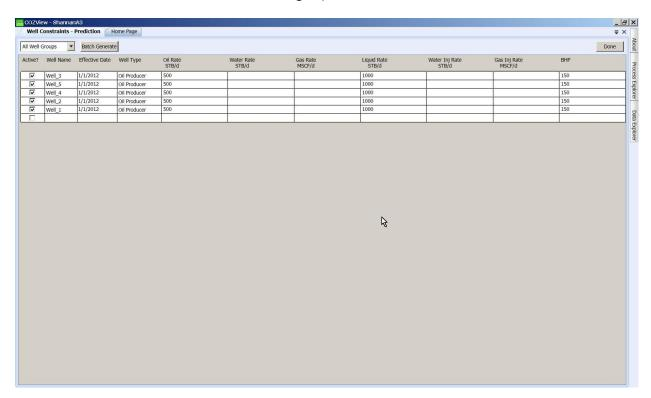
The user may change the well constraints with time by repeating the process at a different date for the affected wells.
