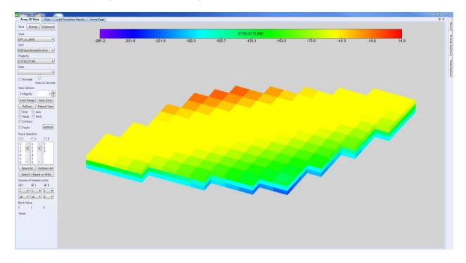
Fence diagrams of any of the property displays can be created in the Fence Selection area. Checking the J box and picking row 3 will provide the display below
