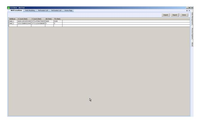
The user can input any missing data and change any data already provided by clicking on the appropriate *Well Name*. The entire well line will be highlighted in blue. The user can then double-click the data field to be input or changed.
