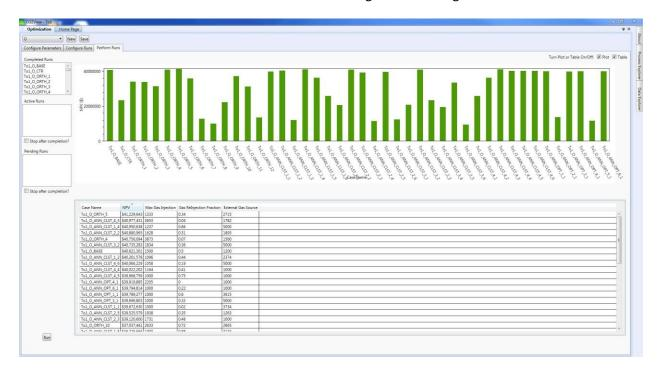
Since the Optimization runs will only have saved field plots and not individual well plots or arrays, the user can select a Case and rerun it as prediction case. The prediction run will provided individual well plots and result arrays.
