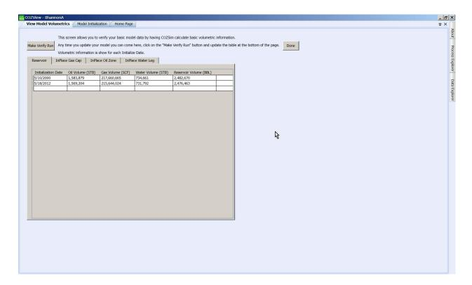
The user may also choose to make adjustments to the static model/formation properties in order to alter the calculated initial in place volumes. If formation properties are changed, but the model initialization parameters are not changed, the user can return to the *View Model Volumetrics* window and select Make Verify Run to recalculate the initial volumetrics.
