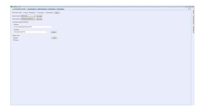
Select *Load* to load results into **COZView** for display from the *Simulation Results* area in Process Explorer.
