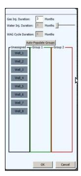
The user can assign the wells to groups by dragging each well from the *Unassigned* column to one of the *Group* columns. Typically, wells are grouped based on surface facilities and/or pattern requirements.
