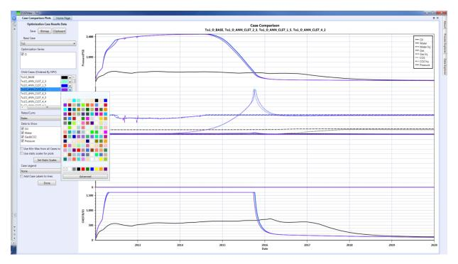
The *Case Legend* can be selected to be at four different places on the plot (i) Lower right, (ii) Upper right, (iii) Lower Left and (IV) Upper left. Selection of the box "Add Case Labels to lines" will add case names to each plot curve.
