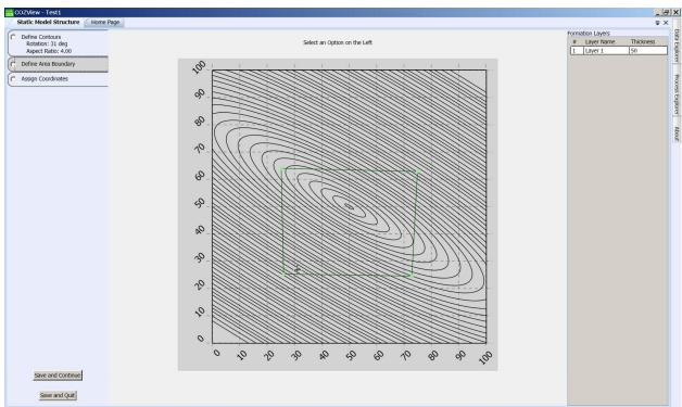
Should the user wish to change a boundary control point, a right-click on the control point will allow that point to be deleted or all points to be deleted. The user can reset the desired control points with appropriate left mouse clicks.
