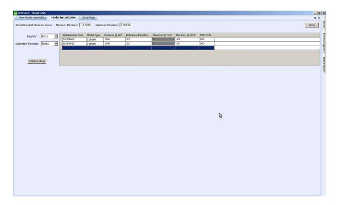
In this example, the difference in Pressure@Ref between the two initialization dates results in different in place volumes.
