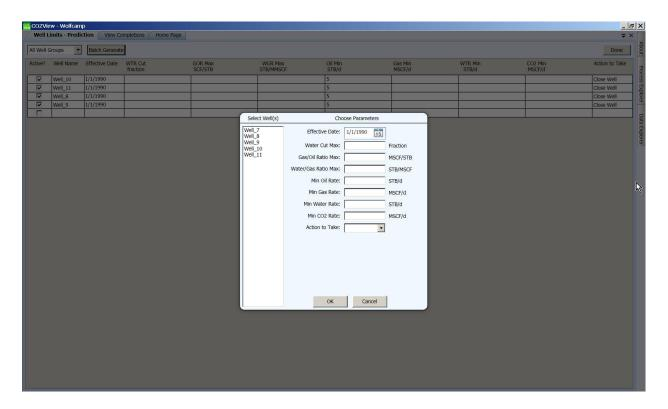
The user must select the appropriate wells, define the activation date, and specify the appropriate limits. Selection of **OK** will generate a table of the well limits for all selected wells. Parameter values for any given well can be changed by selecting the appropriate data field and inputting the new value.
