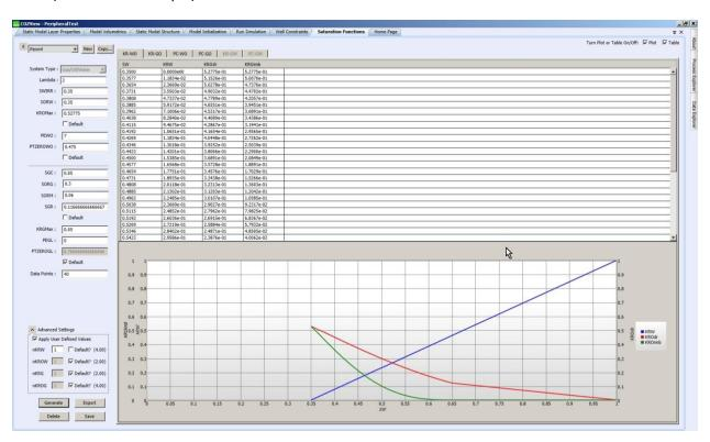
The user can toggle between the Default value and the user defined value by checking and unchecking the *Apply User Defined Values* check box. When the appropriate relative permeability curves have been generated, select **Save**.
