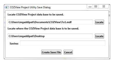
The user must then select the location for the saved file. Select **Create Save** file. A completion window pops up when the process is completed.
