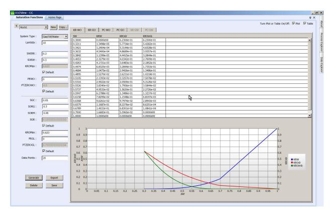
The screen above has generated the saturation function using the default values for all parameters. The screen below is the result of changing only the SWIRR value from 0.3 to 0.4 and generating new curves.
