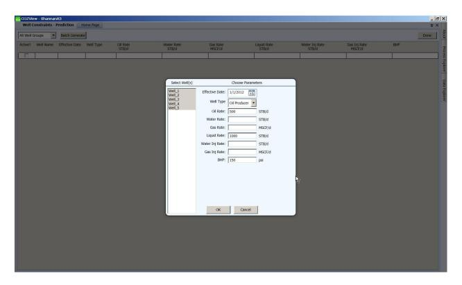
Selection of **OK** will generate a table for all wells selected. Parameter values for any given well can be changed by selecting the appropriate data field and inputting the new value. (A left-click on the data row and a left-click on the data field to be changed.)
