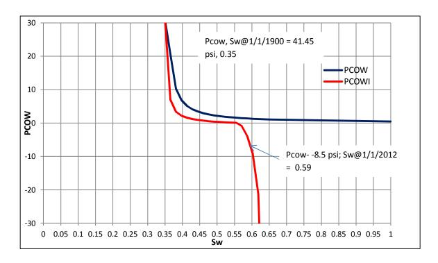
For this example, a PTZEROWO value of 0.57 is appropriate to match the OIP of 1.71 MMSTB. (It is suggested that the number of data points be increased from the default of 20 to 40 during this exercise. This will better display the imbibition curve and the PTZEROWO point.)
