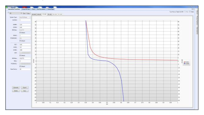
Note that the scale of PCOW (y-axis) is -60 to 60. The capillary pressure calculated at the midpoint of the reservoir is 41 and -8 psi respectively for original and current conditions. PCOW at Midpoint at 1/1/1990 should always be much greater than the highest value on the PCOW scale to assure that the Sw = Swirr. (This PC-WO curve (scale) would suggest a Sw value of approximately 0.37 at the midpoint of the reservoir which is greater than Swirr.)
